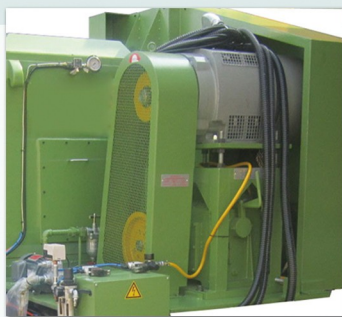
4/8極馬達搭配三段變速(標準) Gear box with 4/8 pole motor for 6-step speed change. (standard)
