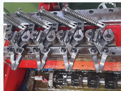
彈簧式夾仔台(標準) Spring transfer mechanism for quickly and securely gripping blanks. (Standard for small models.)
