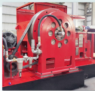
離合器可蓄能便於吋動，變頻器 可無段變速調整(選配) Air clutch for retaining the fly wheel power when performing jog function. (Optional)
