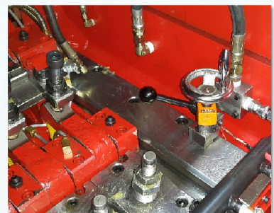
擋料手輪調整(選配) Stopper length adjusted by hand-wheel. (Optional)
